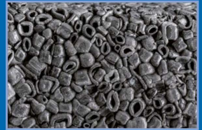
C- or macaroni shaped beads for noise reducing applications
